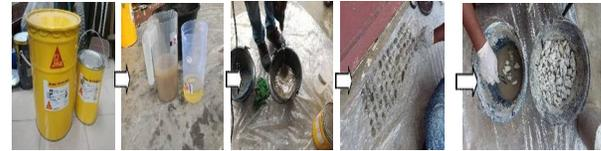
Figure 3: The Method of Applying Resin and Hardener Mix to Recycled Aggregate.
